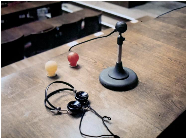
Figure 2: The speakers' equipment—a headset, a microphone, and two light bulbs to signal the requests of the interpreters.
